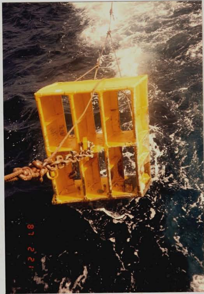
Photo. 6 Paravane otter-board shooting from M.V. PAKNAM
